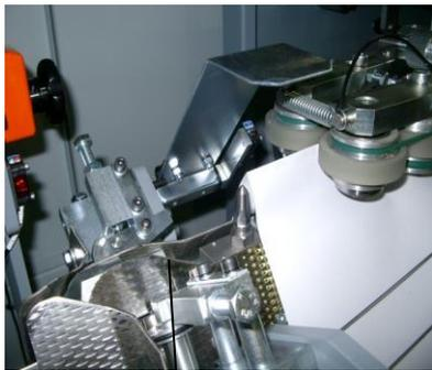
ISG Cold-Glue Application Nozzle on the Smart-binder
